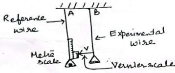
The experimental wire (B) is of uniform area of cross-section also carries a pan in which known weights can be placed. The vernier scale is attached to a pointer at the bottom of experimental wire B and main scale is fixed to the reference wire A.
